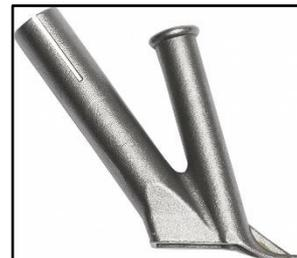
Set the welding machine to approx. 450°C. Use a 5.0mm speed welding nozzle to insert the fusion wire.
