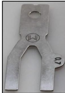
While still warm, push off half of the fusible link with the "Mozart" push-off knife with spacer plate (0.7mm). Allow the remaining, excess fusible link to cool completely and then push it off flush with the surface of the floor covering using the "Mozart" push-off knife without spacer plate.
